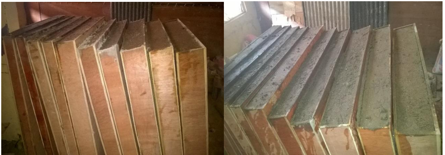
Plate 3: Cross section of sawdust-crete laminated composite slabs.
