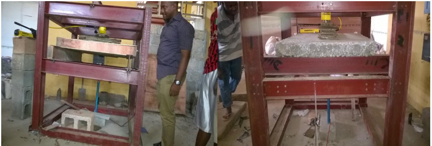
Plate 2: Arrangement of slab during crushing as required by BS EN 12390 [24].
