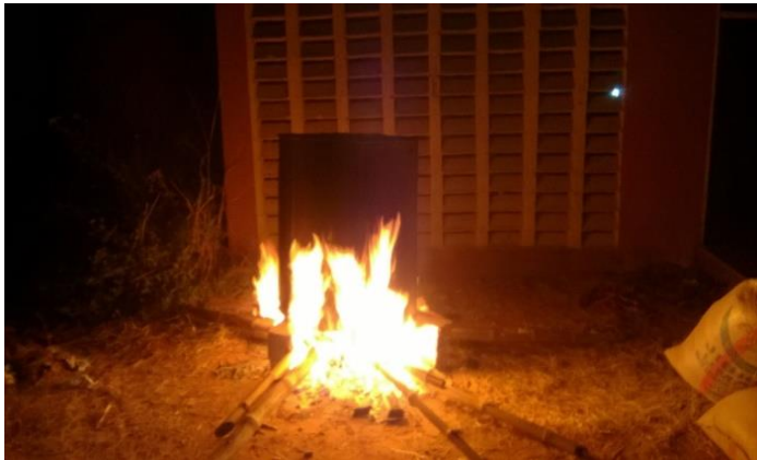
Plate 1: Boiling of Sawdust to remove any Resin for proper bonding.
