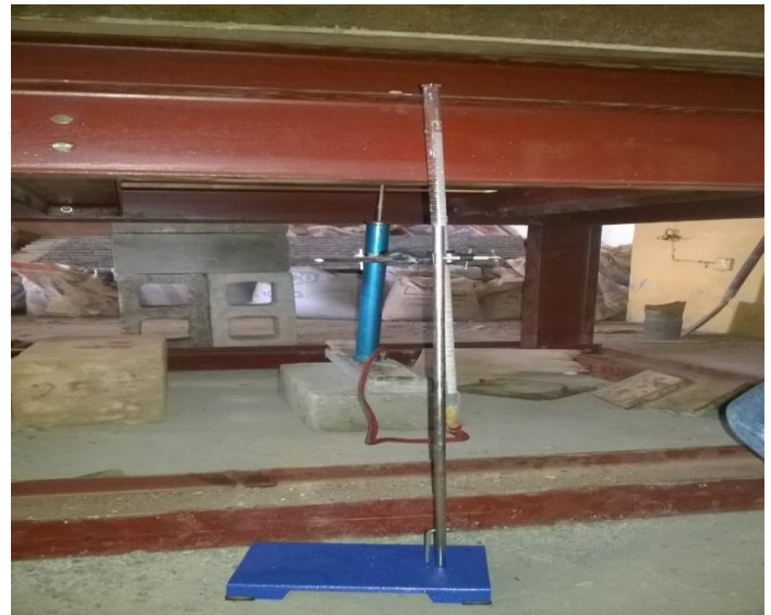
Plate 4: Deflection measurement using principle of incompressibility of water
