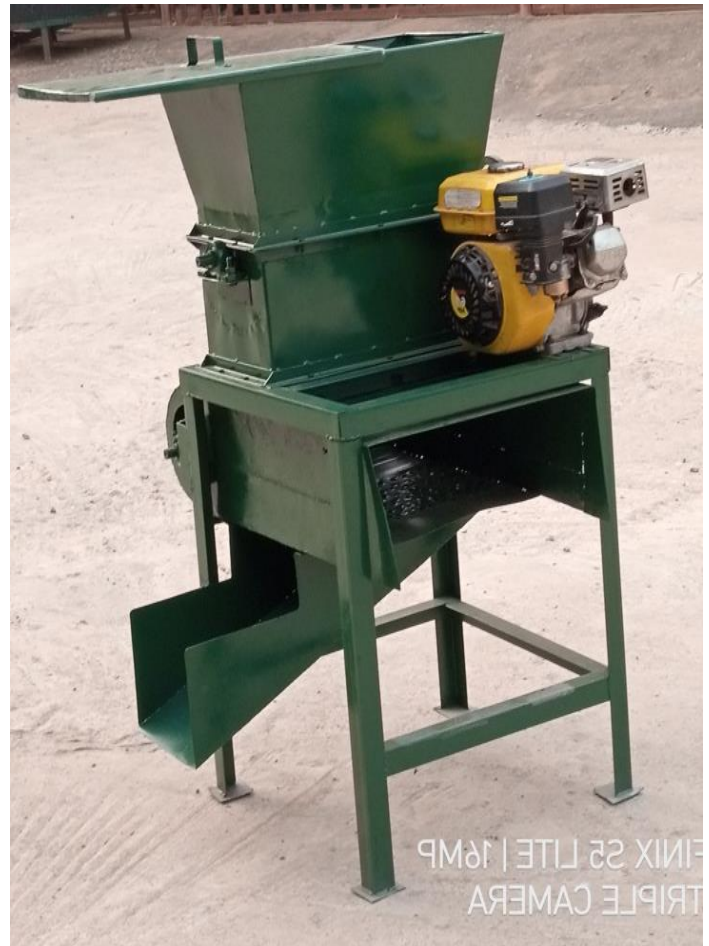
Figure 1: Developed Cowpea Thresher
