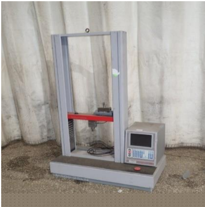
Fig. 3: Experimental set up using Instron Universal testing machine
