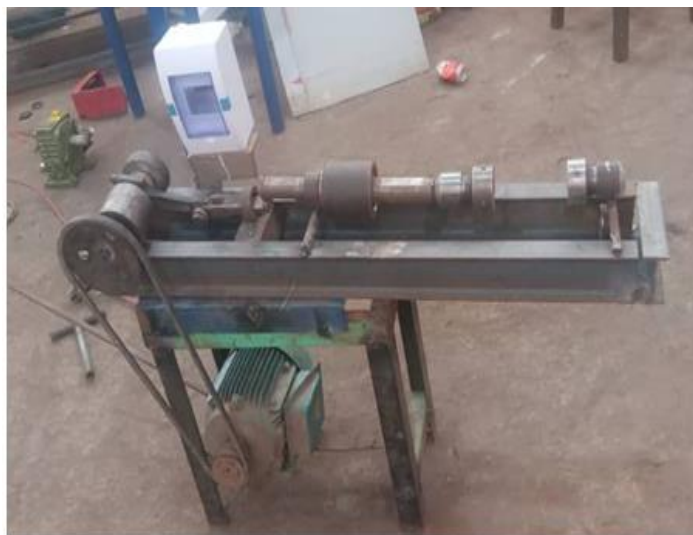
Figure 6: Fabricated Fatigue Strength machine
