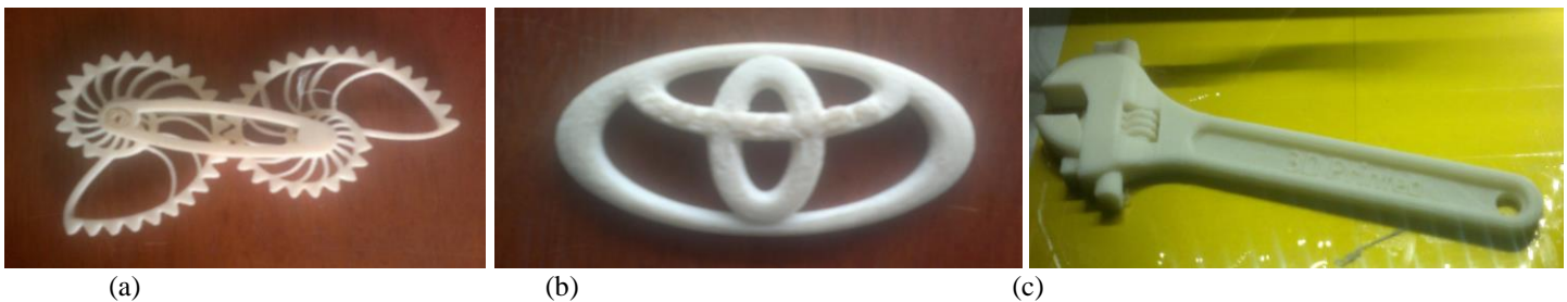
Figure 9: Printed artefacts and components: (a) a Nautilus gear assembly; (b) a Toyota car logo; (c) an adjustable wrench
