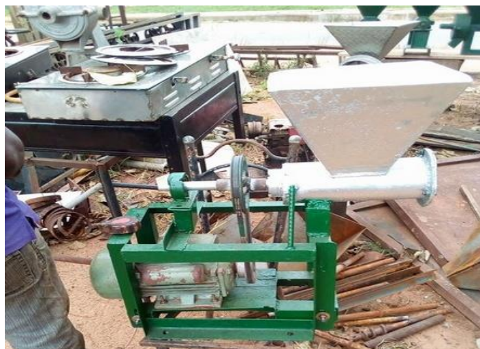
Plate 1: Pelletizer after fabrication at a local workshop
