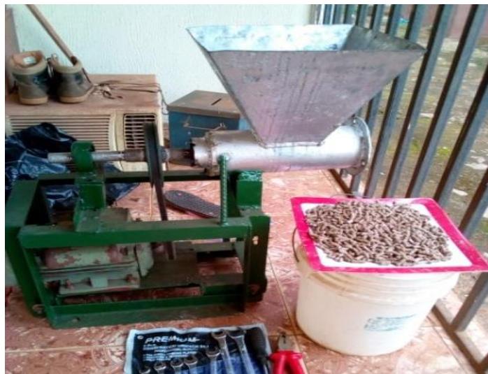
Plate 2: Pelletizer and NPK fertilizer pellets produced
