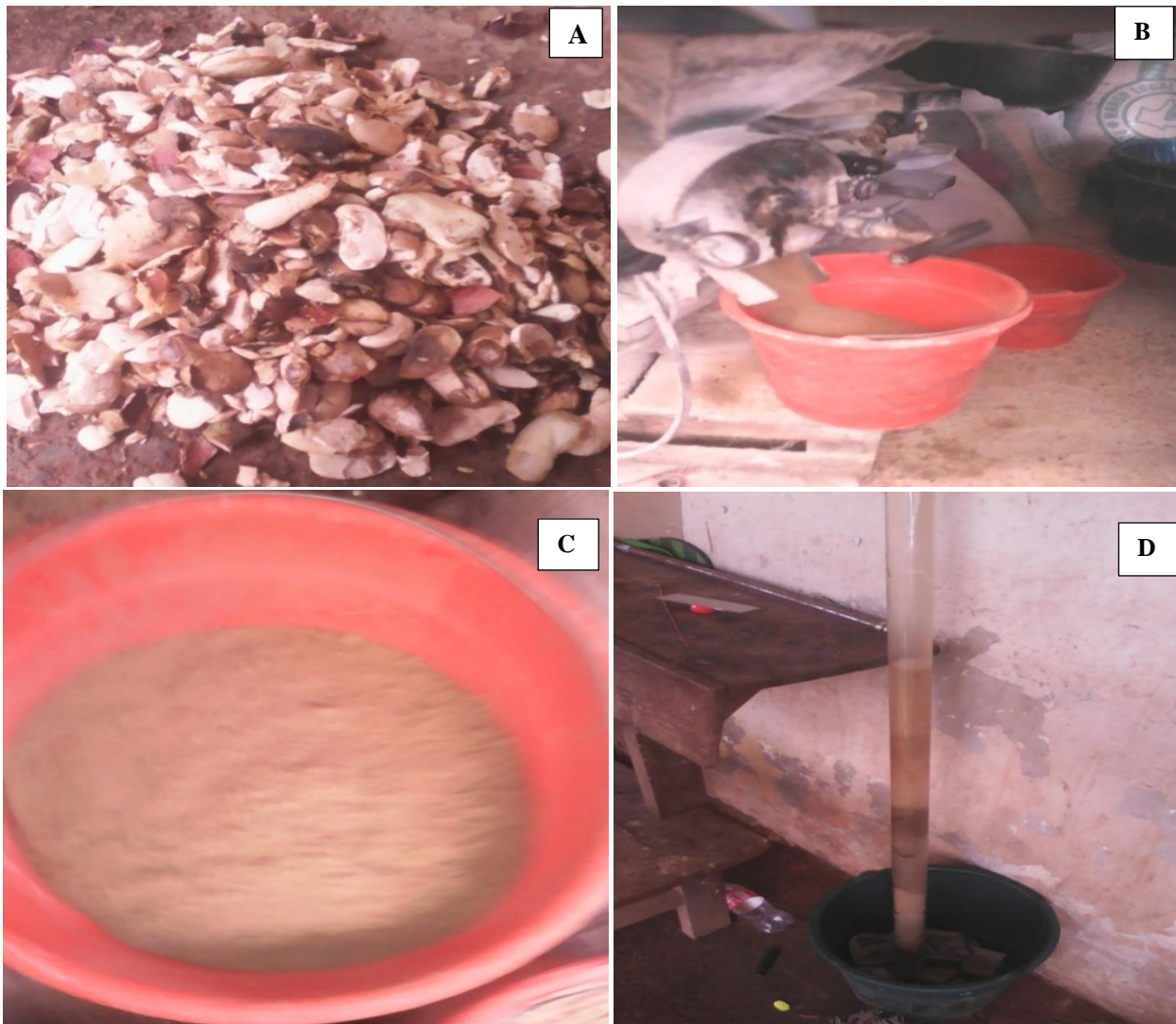
Figure 2: (a) Mango seeds (b) Mango seeds processing (c) Grinded mango seeds (d) Burette setup for separation of biodiesel from glycerin
