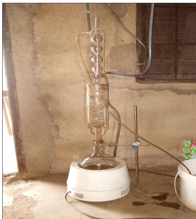
Figure 1: A Soxhlet Oil Extractor ([22])
