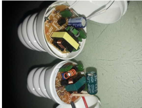
(a) Electronic Ballast of the 11W and 15W CFLs
