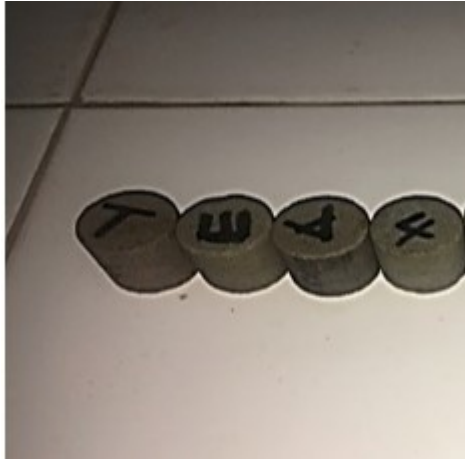
Figure 1: Sandstone Core Samples.
