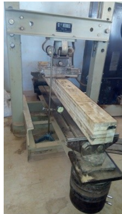
Figure 3: Two points static bending test setup.
