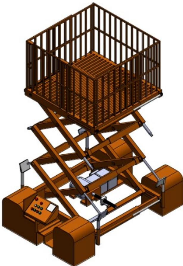
Figure 18: Isometric view of the designed enhanced intelligent mobile scissor lifting system in full lift position.
