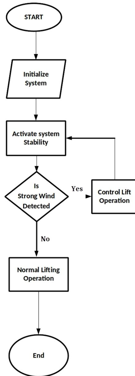
Figure 5: Flow chart for the the enhanced intelligent mobile scissor lifting system.
