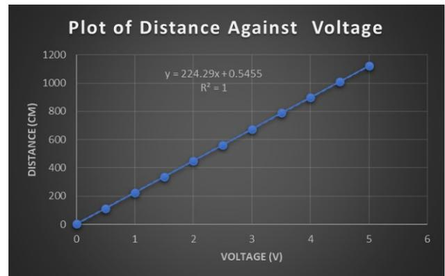
Figure 12: The simulation plot of the distance against voltage for the enhanced mobile scissor lifting system.
