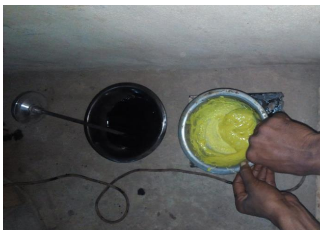
Figure 2: Pure Bitumen and DFP Dissolved in kerosene
