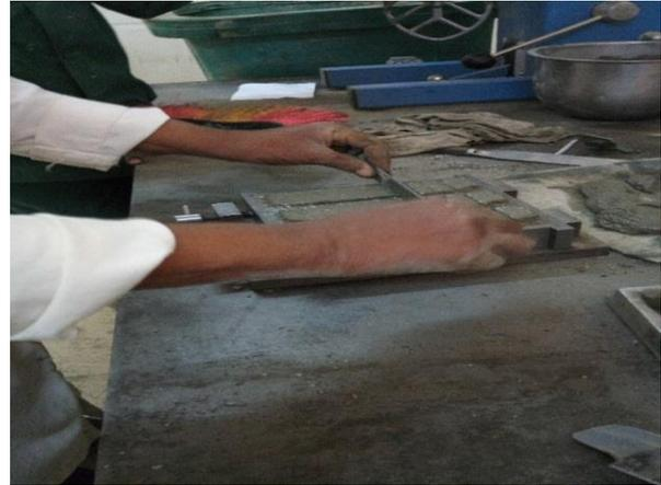
*Plate I: Moulding of the Mortar Prisms**Table 3: Cement Mix Composition used in the study*
