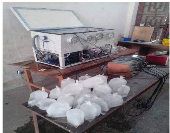
Plate 4: Ice blocks formed within 6 hours of running the sub-cooled system
