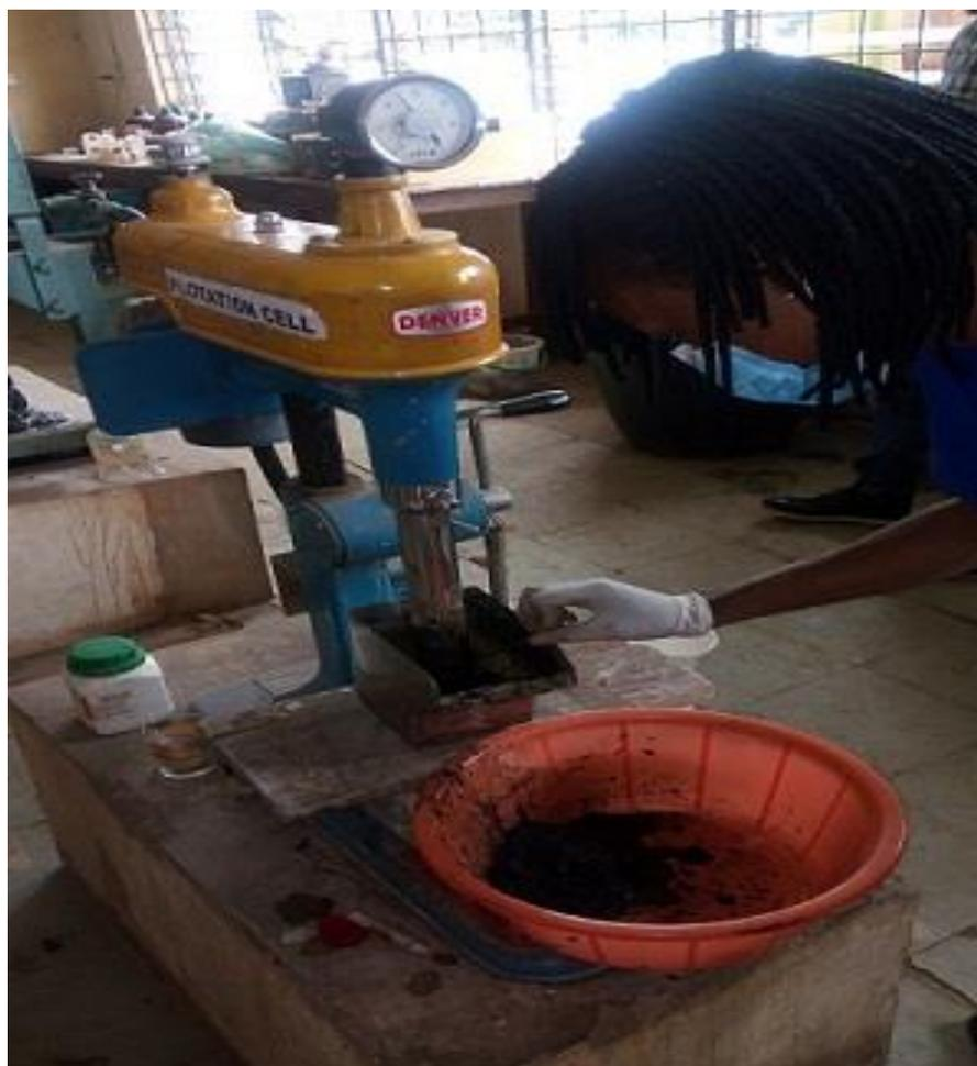
Plate 1: Denver Flotation Cell
