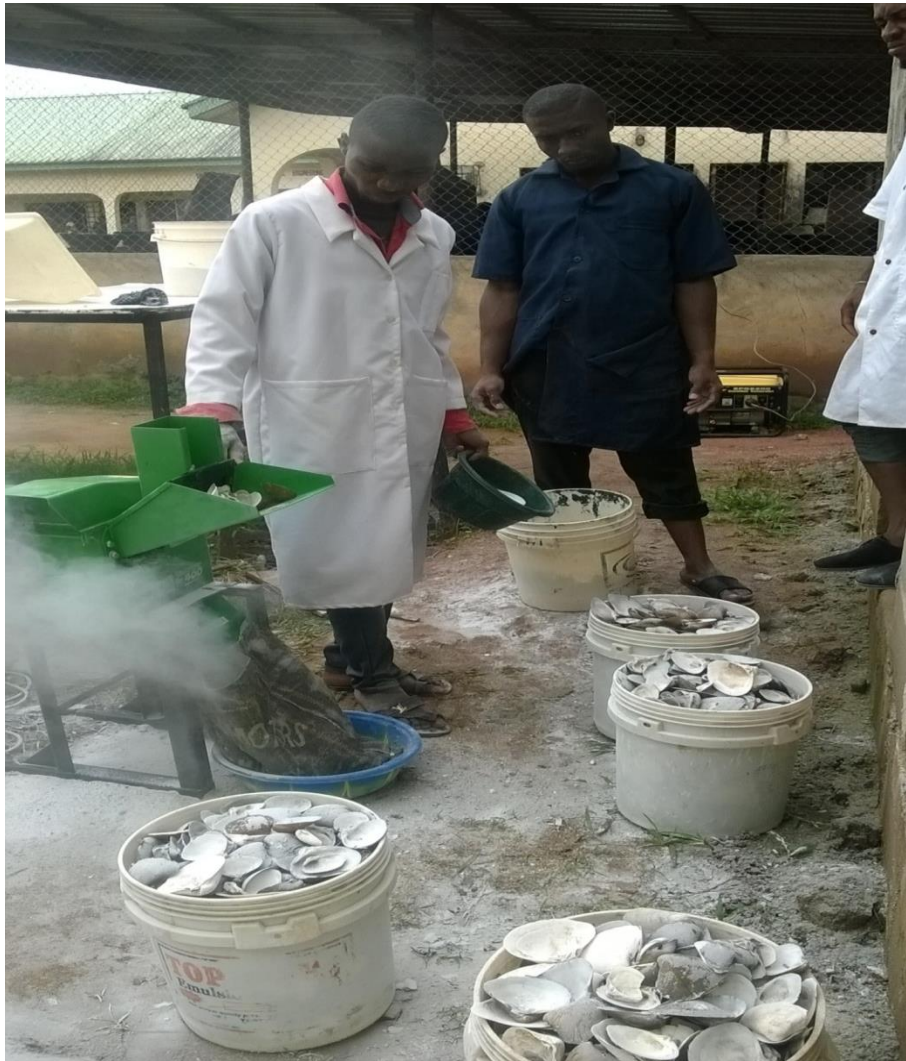
Fig 2: Oyster Shells undergoing Crushing by Hammer Mill Machine
