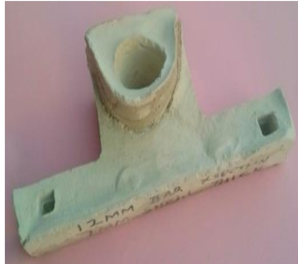
Fig 5: Shell produced after burning of polystyrene and firing
