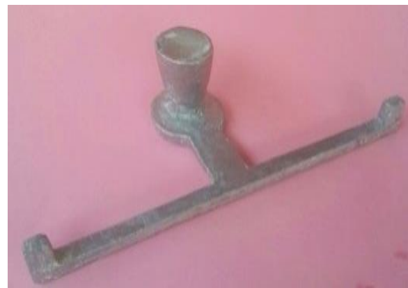
Fig. 6: Bar casting after knockout and cleaning operation
