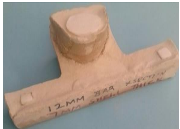
Fig. 4: Bar shell formed and left for drying
