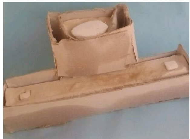
Fig. 3: Strawboard box temporarily housing the pattern and the poured slurry
