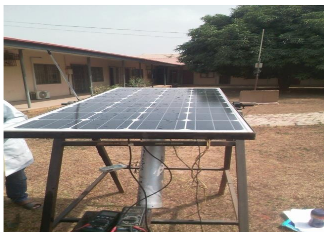
Figure 1: View of the experimental set up without water cooling
