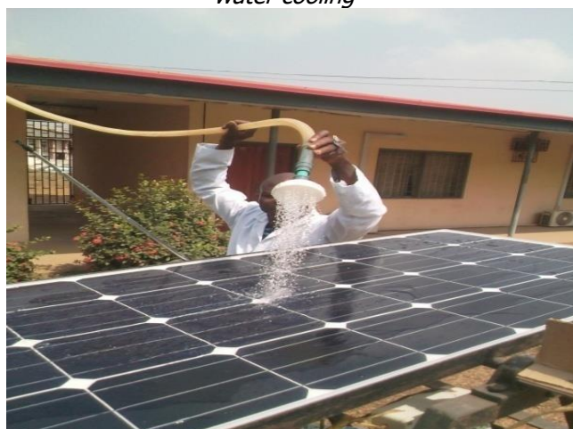
Figure 2: View of the experimental set up with water cooling.
