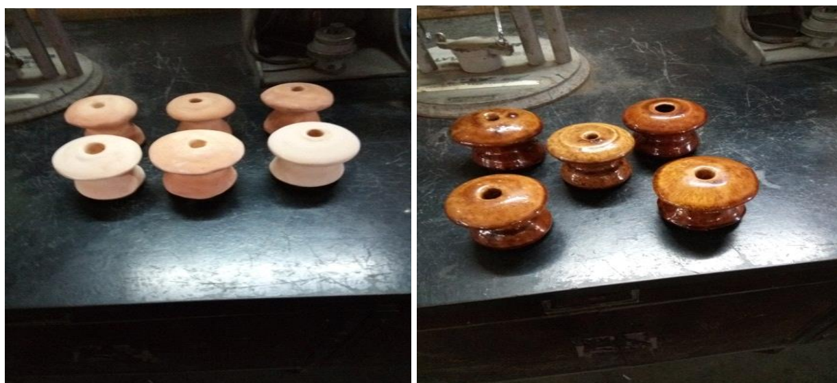
Figure 1: Pictures showing different shackle insulators in their (left) bisque fired state and (right) sintered and glazed state.
