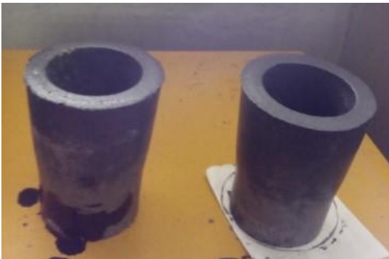
Plate 1: Produced Clay bonded Graphite Crucible
