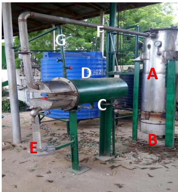
Plate 1: Steam Distillation Pilot Plant for Extracting Essential Oil from Lemon Grass
