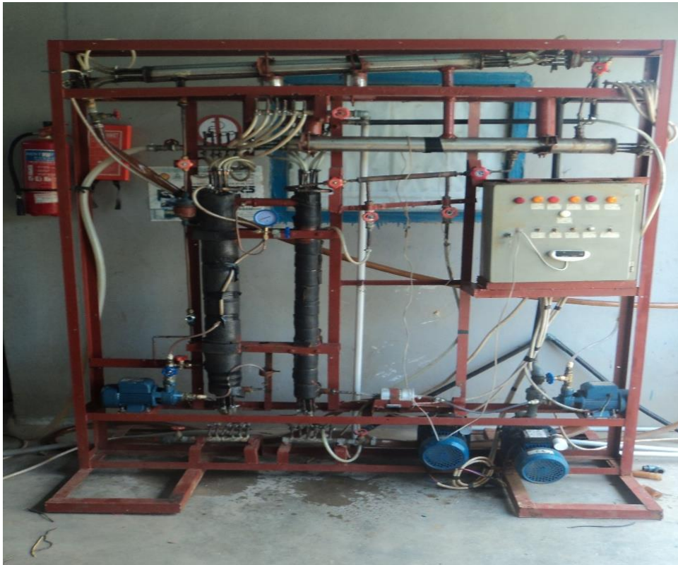
Figure 3: The 3 kW absorption chiller prototype
