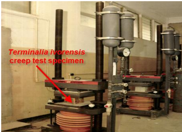
Plate 1: Set-up of Creep Testing Machine with Specimen Under Loading
