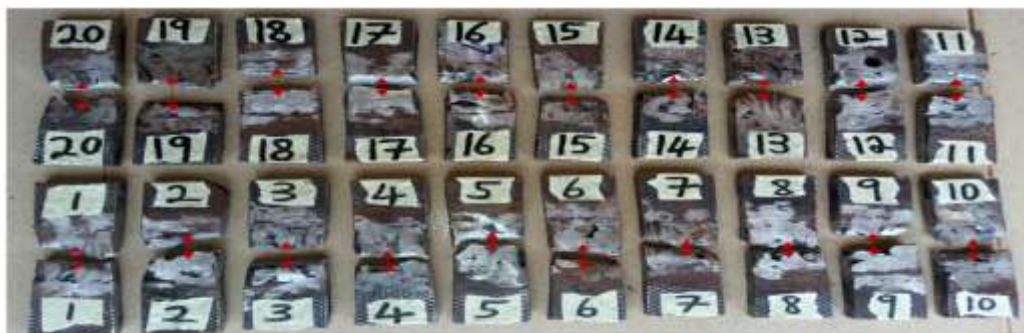
Figure 1: Samples Subjected Tensile test showing the Breaking Point
