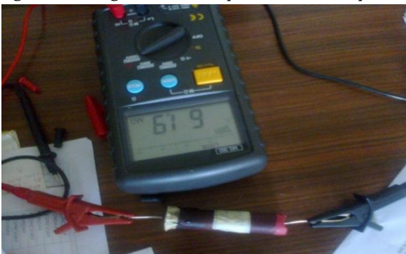
Fig. 3: Experimental Set up Showing the Determination of Resistivity using Digital Mega Insulation Tester. MS 360.
