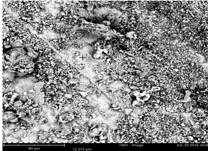
Fig. 11 SEM photograph of the tempered sample at 550 °C after 90 days immersion in 1M NaCl solution
