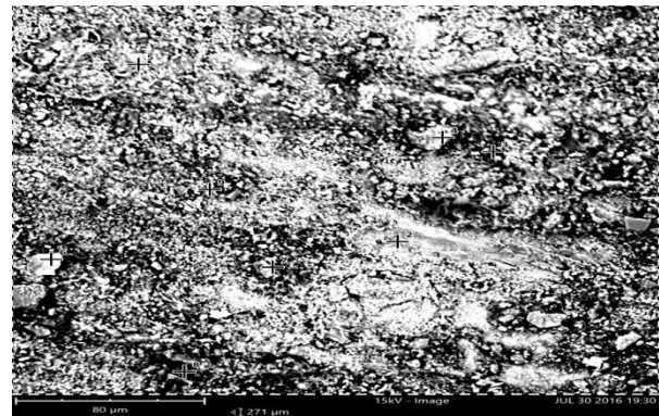
Fig. 8 SEM photograph of the tempered sample at 250 °C after 90 days immersion in 1M NaCl solution
