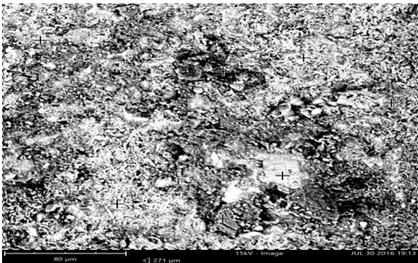
Fig. 7 SEM photograph of the control sample after 90 days immersion in 1M NaCl solution
