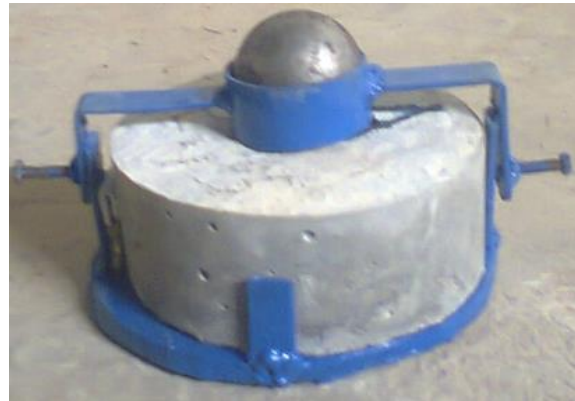
Plate 5: Test Setup for Impact Test
