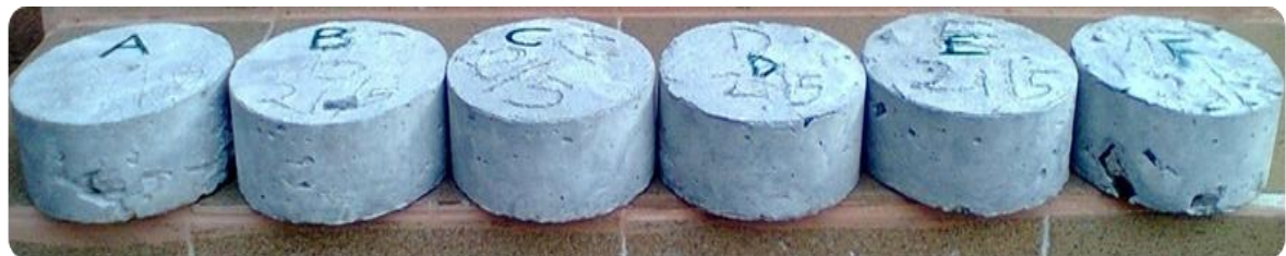
Plate 6: Circular Disc Concrete Specimen
