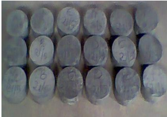
Plate 4: Circular Discs Samples for Impact Test
