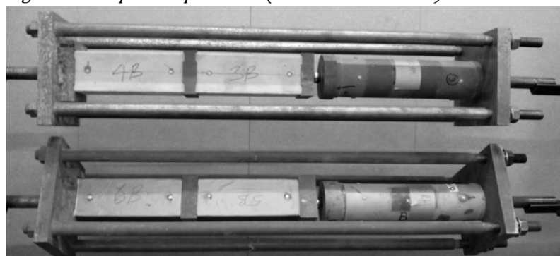
Figure 2: Compressive creep rigs showing sealed and unsealed specimens
