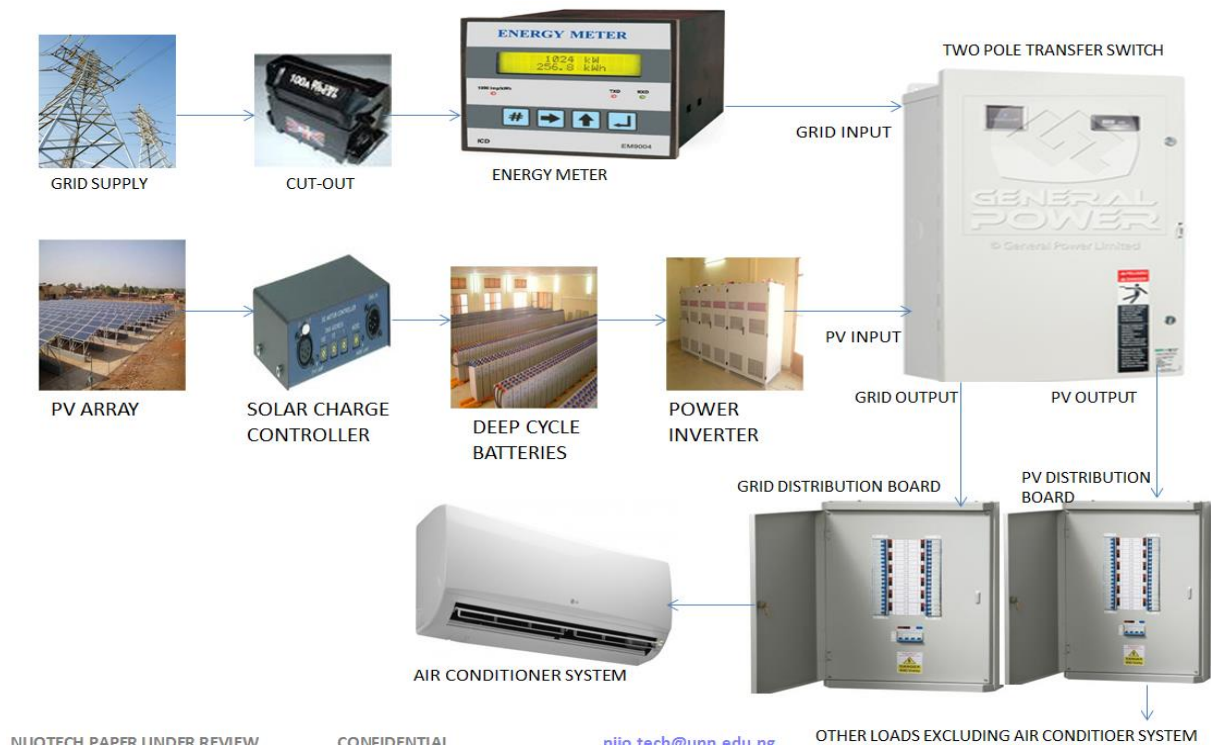
Figure 17: Block Diagram of the Proposed PV- Grid Connection for the Building
