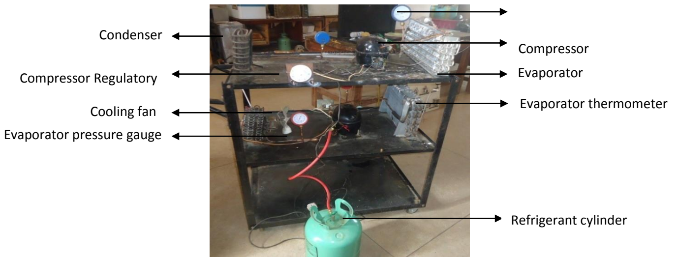
Figure 1: A typical setup for investigating the coefficient of performance of the refrigerants
