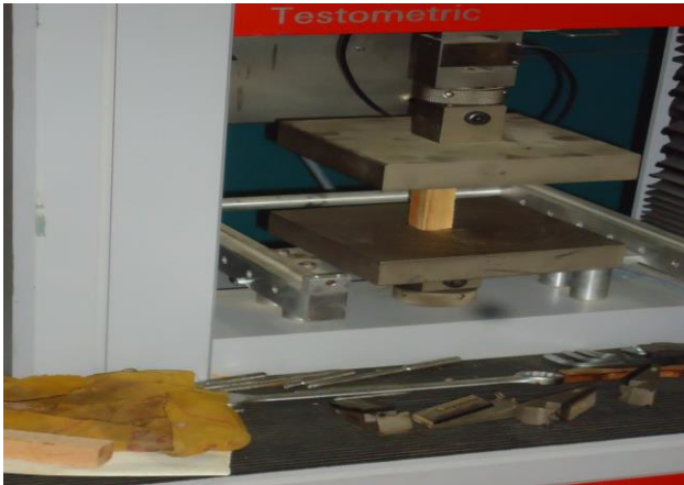
Plate III: Compression test set up
