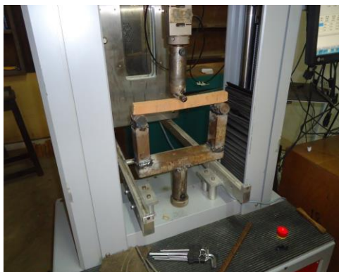
Plate IV: (a) Bending strength test set-up
