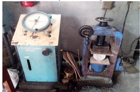
Plate 2: Avery Denison Universal Testing Machine
