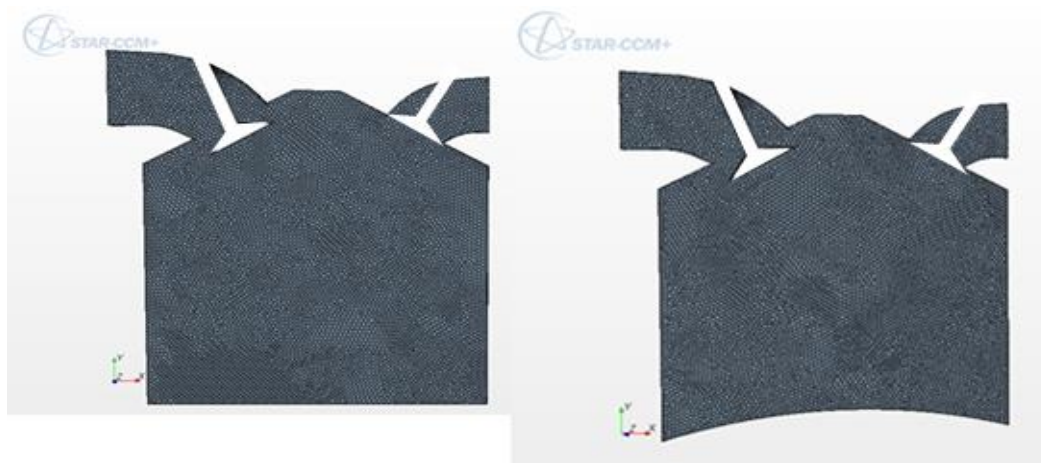
Figure 4: Infinitesimal mesh for both piston models
