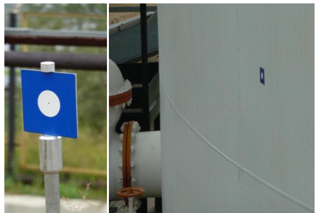
Figure 1: Terrestrial laser scanner Targets
