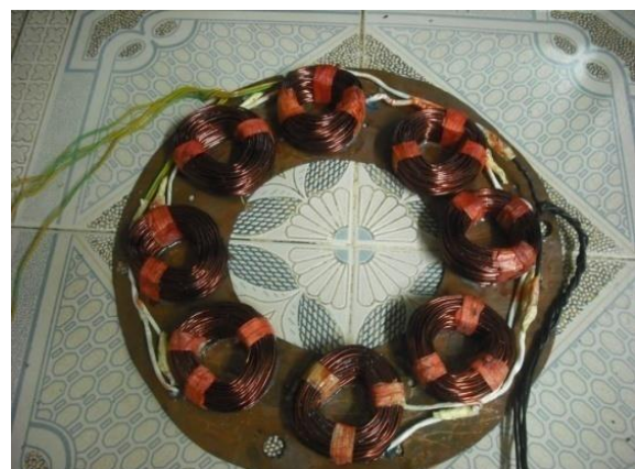
Fig.5: The developed Concentrated Air-Cored Stator Winding
