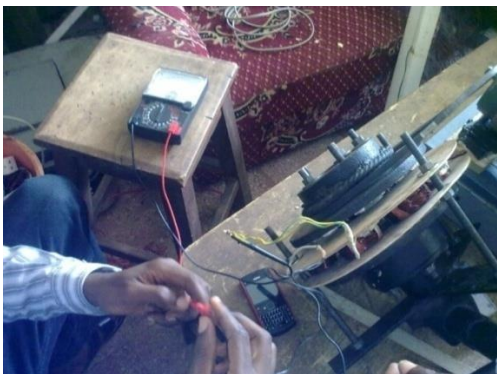
Fig. 8: Test Set-Up for the developed AFPMA
