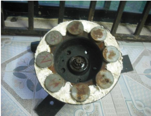
Fig. 7: Permanent magnets as mounted on the rotor plate
