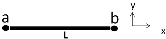
Figure 7: A beam model with length L and nodes a and b
