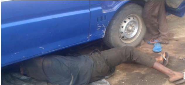
Plate 5: Automobile mechanic working beneath with limited clearance and awkward posture
