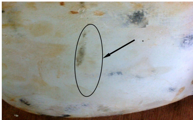
Figure 8(a): Color lightening of bumper surface after impact test with complete restraints
