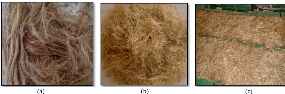
Figure 1: Lalloh Plant Fibre (a) – extracted, retted, scoured and dried fibres, (b)-Chopped fibre strands, (c) – Fibre Mats
