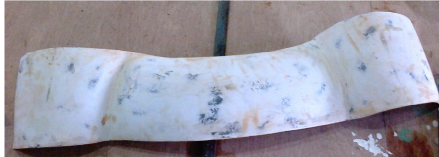
Figure 4(a): Bumper surface after impact test with complete restraints
