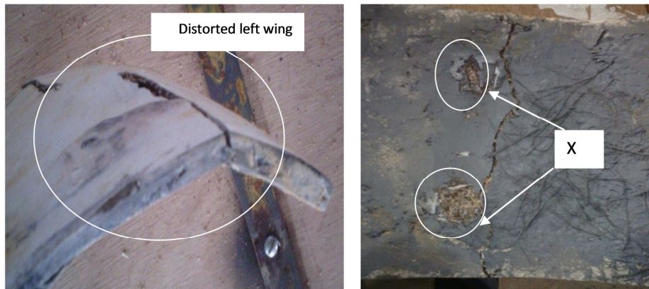
Figure 5: Bumper Displacement and positions of broken off fasteners
