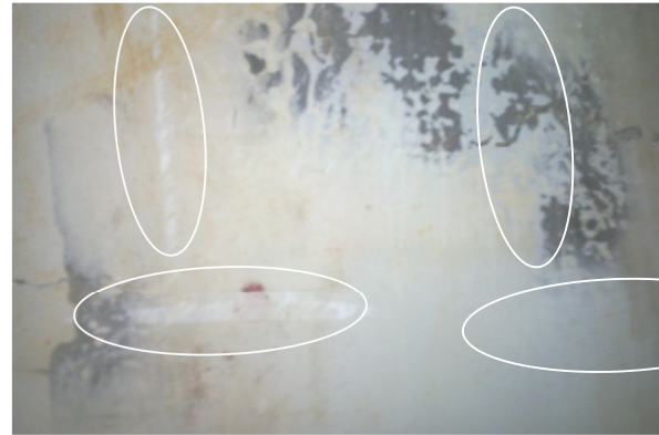
Figure 8(b): Color lightening of bumper surface after test with two-point restraints
