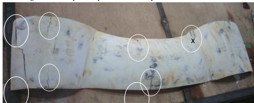
Figure 6: Crashed bumper showing tears more than 1cm
