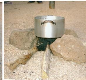
Figure 2: WBT on Metal Shield stove
