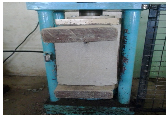
Plate 2: Specimen under Splitting Tensile Load
