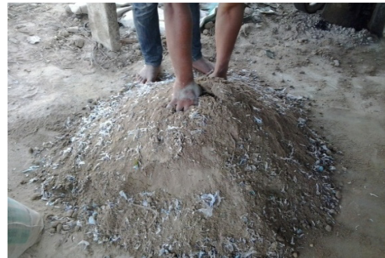
Plate 1: Measured Sand and Shredded Polythene
