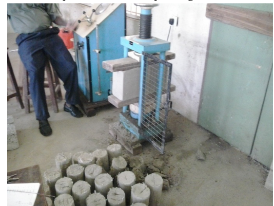
Plate 3: Crushing of Sandcrete Block
