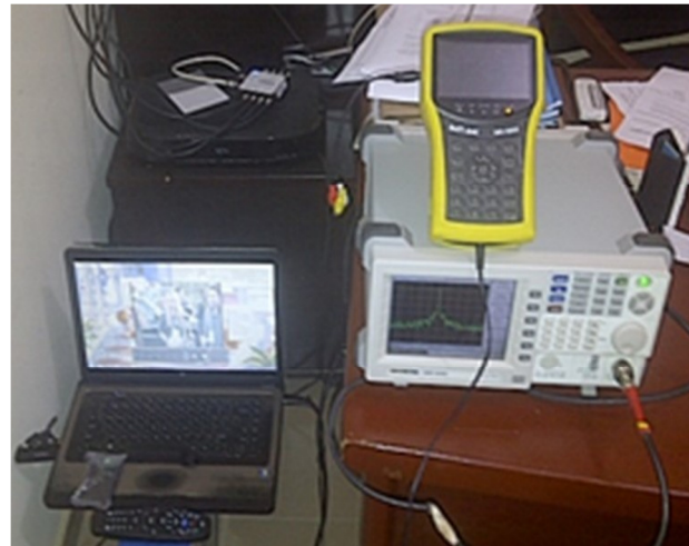
Figure 3. Indoor unit of the measurement system
