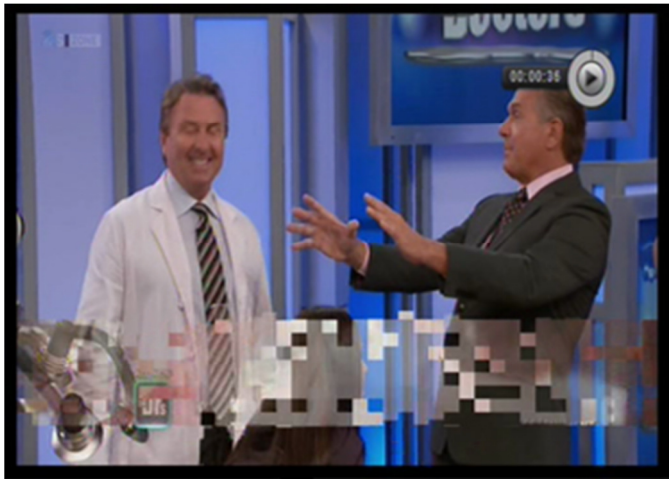
Figure 5. Recorded frame with pronounced pixelation artifact
