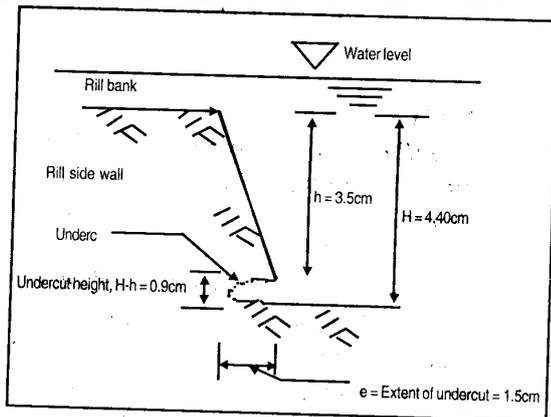
**Fig 1:** Sketch of a half section of a ponded rill bank with undercut
