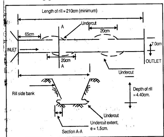
**Fig. 2:** Sketch of the rill indicating undercutting positions.
