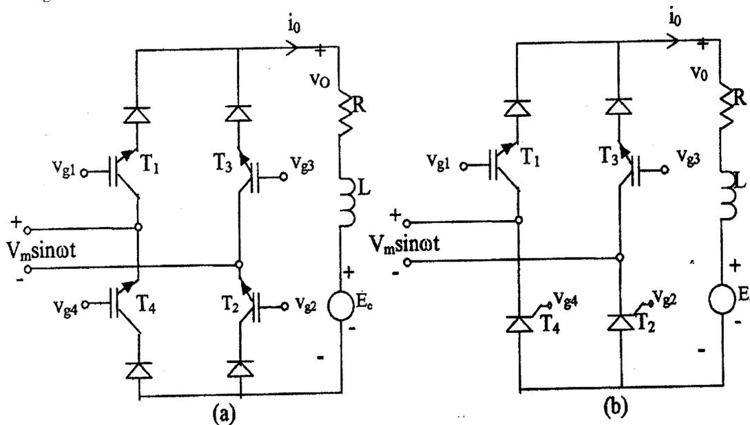
Fig. 1 Illustrative forms of the PWM AC/DC Converter
