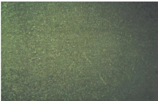
*Micrograph A3: Microstructure of 0.509% carbon steel quenched in engine oil, showing full martensite (dark) x 200.*
