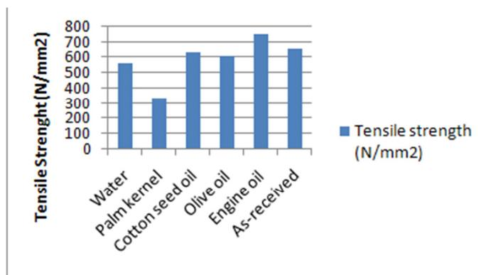
Figure 2: Tensile Strength values of the medium carbon steel sample in different quenchants.
