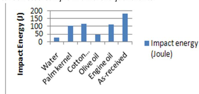
Figure 4: Impact Energy values of the medium carbon steel sample in different quenchants.
