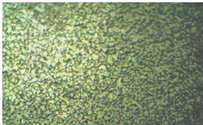
*Micrograph A6: Micrograph of 0.509% steel quenched in olive oil, showing low proportion of martensitic structure (white) with retained austenite (dark).*
