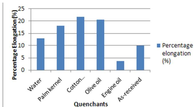
Figure 3: Percentage Elongation values of the medium carbon steel sample in different quenchants.
