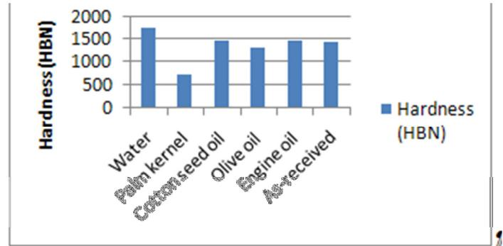
Figure 5: Hardness values of the medium carbon steel sample in different quenchants.
