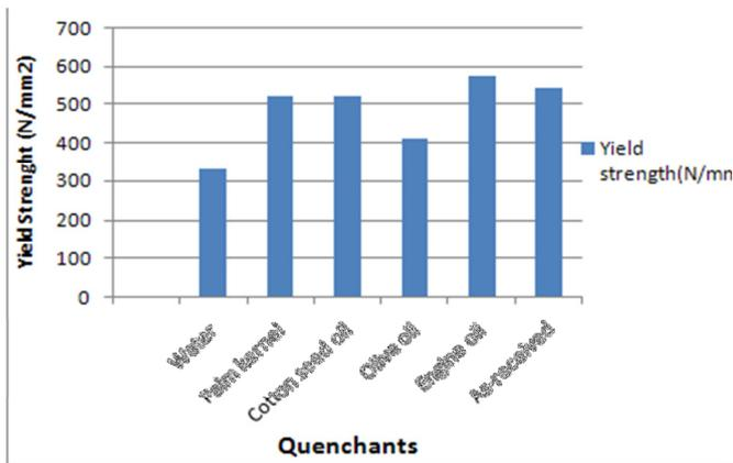
Figure 1: Yield Strength values of the medium carbon steel sample in different quenchants.
