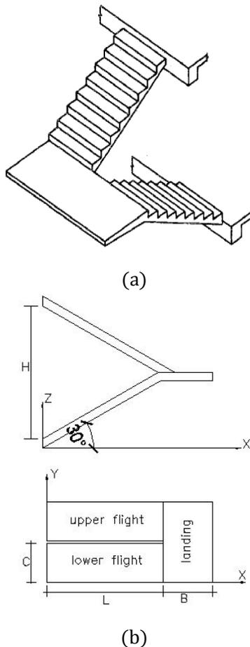
Figure 1: Stair slab geometry, (a) elevation, (b) plan
