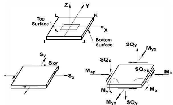
Figure 4: Notations for plate outputs
