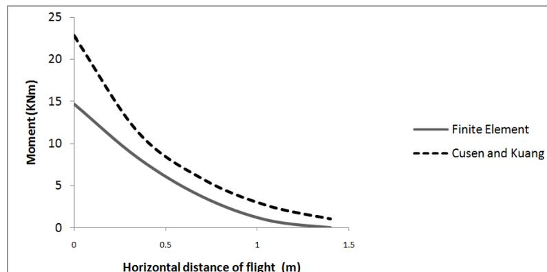
Figure 7: Comparison of Bending Moments at Landing
