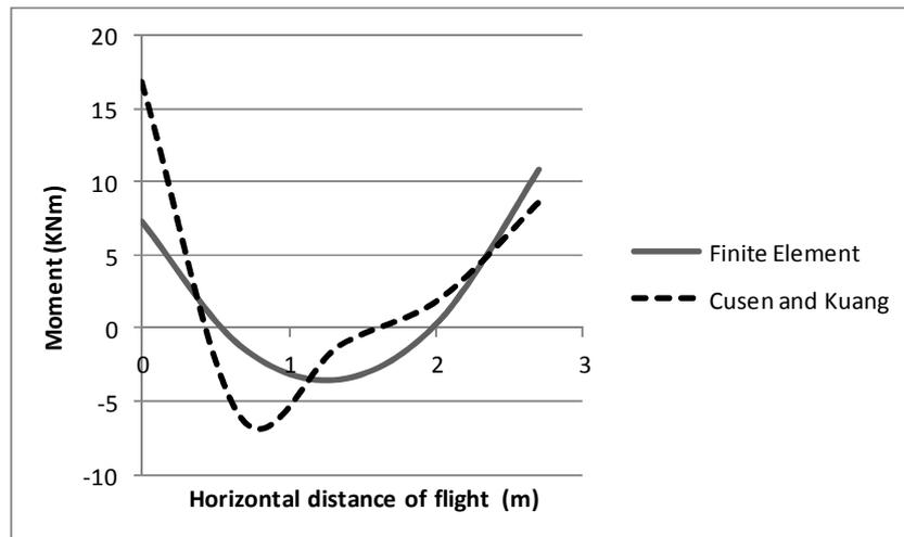
Figure 6: Comparison of Bending Moments of Flight
