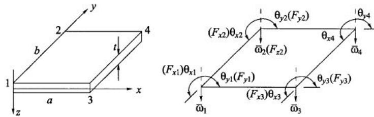
Figure 3: Rectangular Finite Element for Plate Flexure
