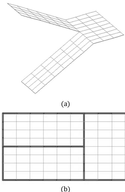
Figure 2: Finite element mesh of the stair way
