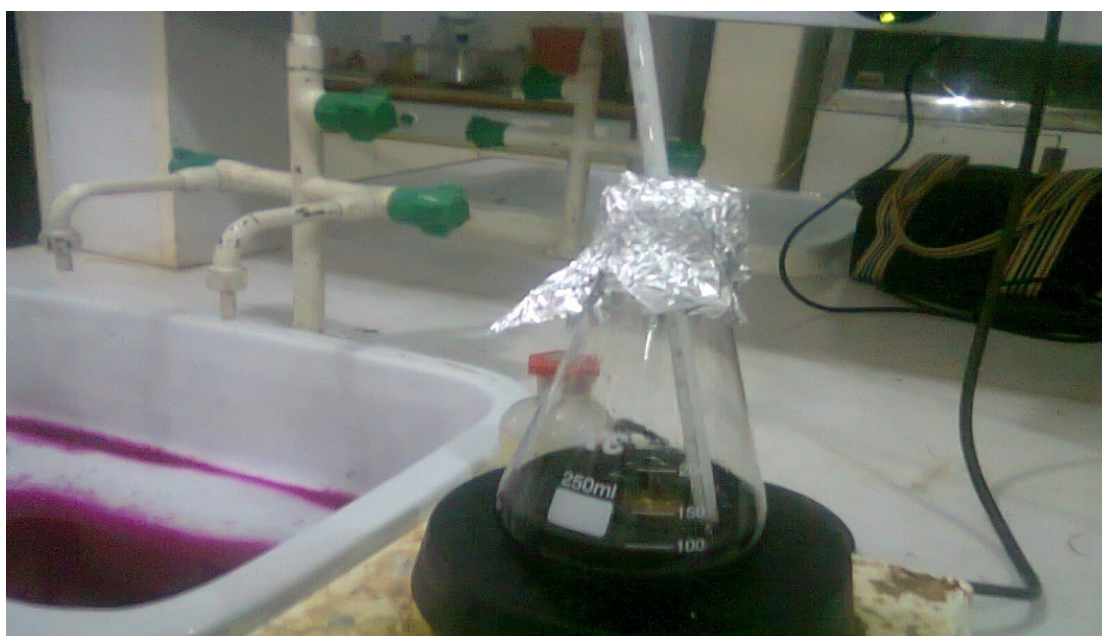
Figure 2: The Esterification/Transesterification Process Setup
