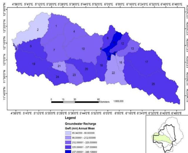
**Figure 11:** Groundwater recharge distribution for the Zamfara river watershed
