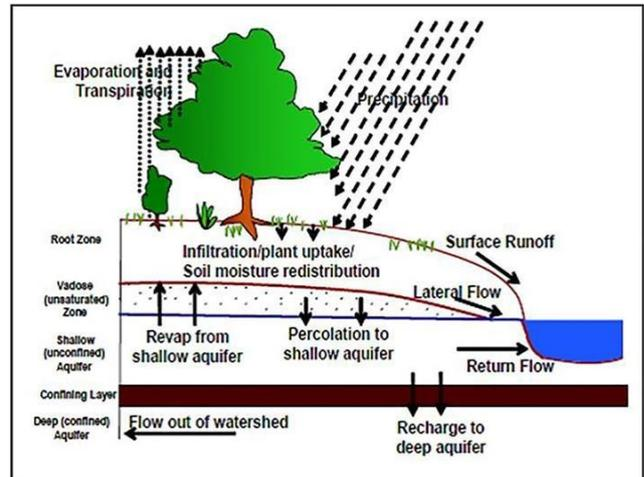
Figure 2: The Hydrological process of the SWAT model [16]
