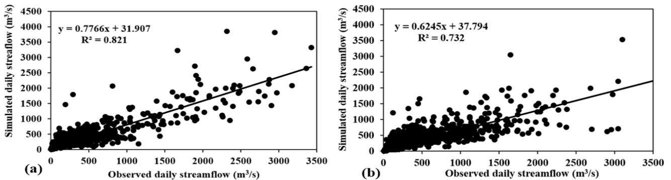
**Figure 9:** Plot of daily stream flow (river) for (a) Calibration period (1993-2021) and (b) Validation period (2001-2021)
