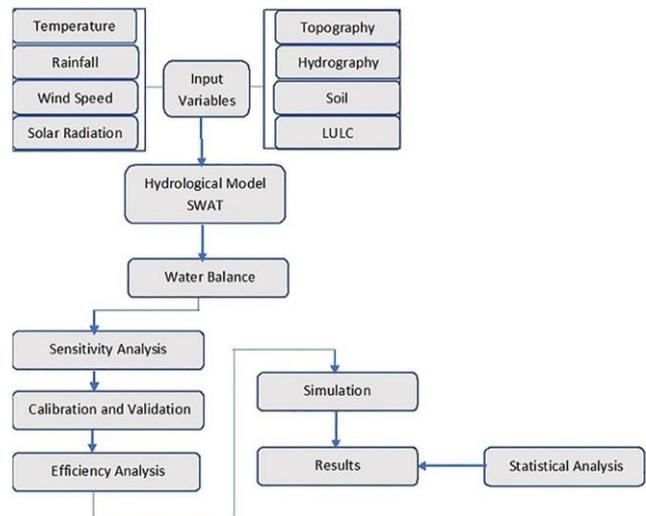
**Figure 8:** SWAT model flow Structure
