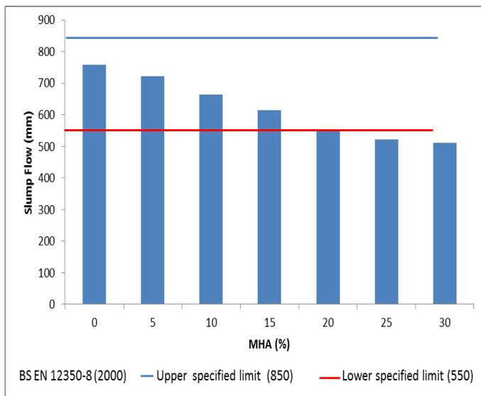
**Figure 2:** Variation of Slump Flow for increasing Millet Husk Ash Content in Self-Compacting Concrete
