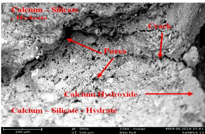
**Figure 11:** Scanning Electron Micrograph of Self Compacting Concrete Specimen containing Optimum Millet Husk Content Sample (5 % Millet Husk Ash) at 28 days Curing Age
