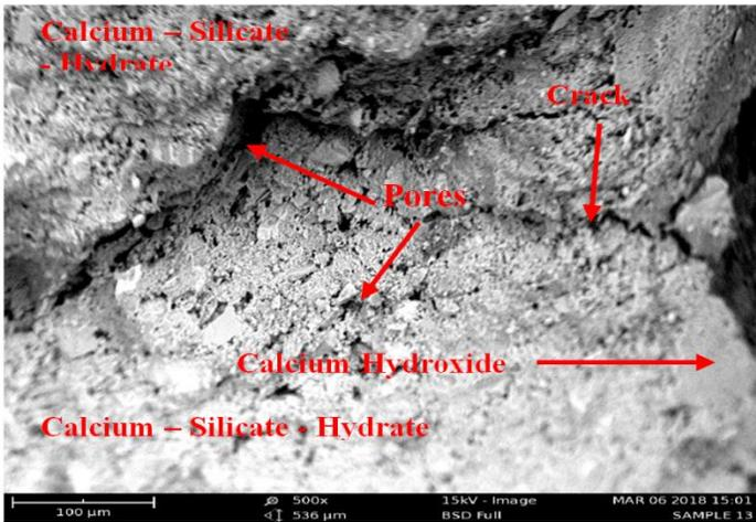
**Figure 9:** Scanning Electron Micrograph of Control Sample (0 % Millet Husk Ash) of Self Compacting Concrete at 90 days Curing Age
