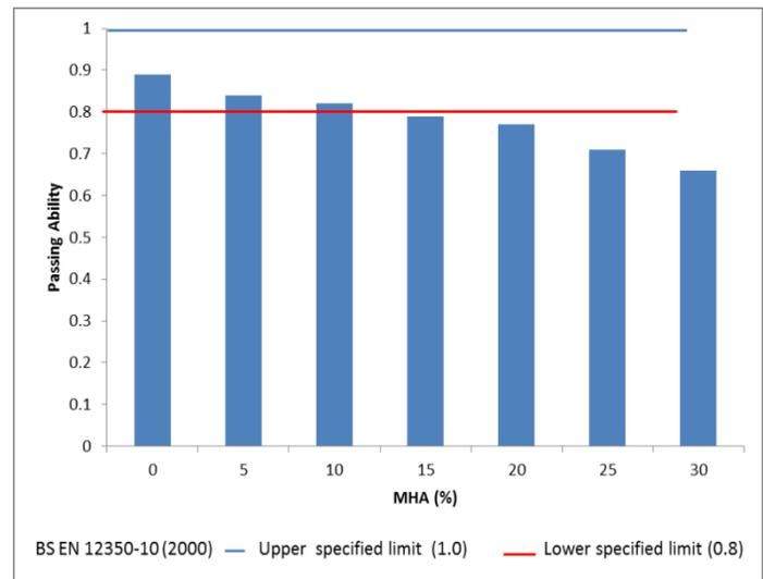
**Figure 3:** Variation of Passing Ability for increasing Millet Husk Ash Content in Self-Compacting Concrete
