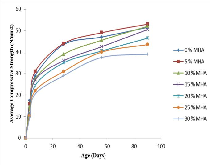
**Figure 5:** Compressive Strength of Self-Compacting Concrete modified with Millet Husk Ash
