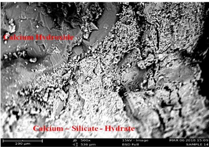
**Figure 10:** Scanning Electron Micrograph of Self Compacting Concrete Specimen containing Optimum Millet Husk Content Sample (5 % Millet Husk Ash) at 7 days Curing Age
