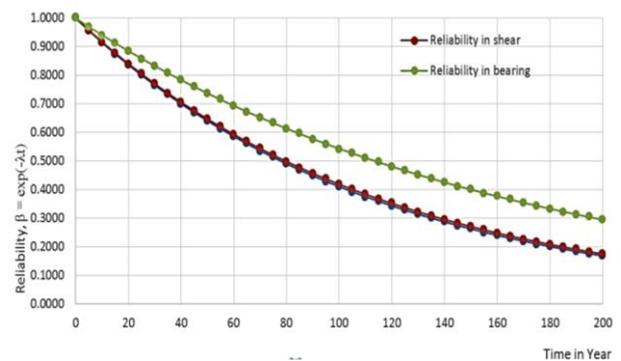
Figure 1: Reliability of *Anogeissus schimperi* Timber Bridge Beam
