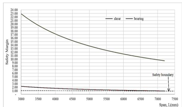
Figure 2 Variation in Span with the Safety Margin of *Anogeissus Schimperi* Timber Bridge Beam
