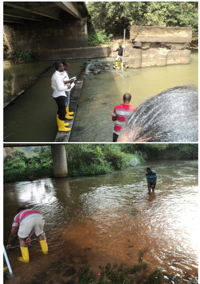
Plates.1 & 2: Measuring discharge of Ovia River
